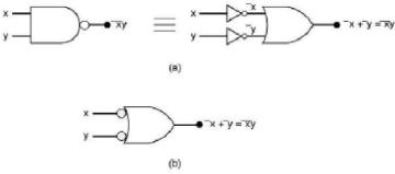
Proof (via Truth Table) of DeMorgan's Theorem  $\overline{A+B} = \overline{A*B}$
